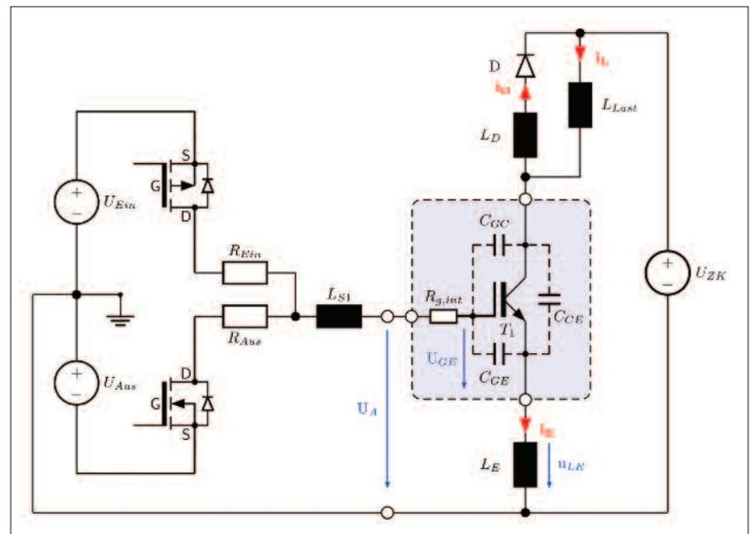
Figure 2: Equivalent circuit diagram with driver connection
