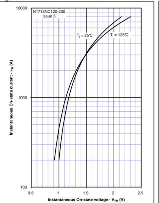
Figure 1 - On-state characteristics of Limit device
