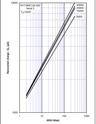
Figure 5 - Total recovered charge, Q<sub>rr</sub>
