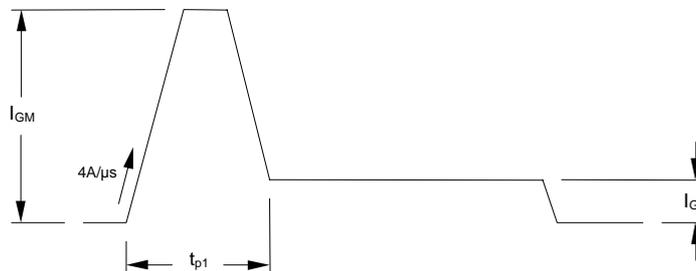
The magnitude of  $I_{GM}$  should be between five and ten times  $I_{GT}$ , which is shown on page 2. Its duration ( $t_{p1}$ ) should be 20μs or sufficient to allow the anode current to reach ten times  $I_L$ , whichever is greater. Otherwise, an increase in pulse current could be needed to supply the necessary charge to trigger. The 'back-porch' current  $I_G$  should remain flowing for the same duration as the anode current and have a magnitude in the order of 1.5 times  $I_{GT}$ .
