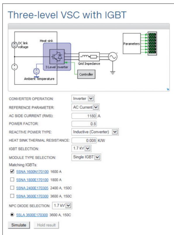
SEMIS offers a user friendly interface for parameter set up and provides a comprehensive steady state analysis for the selected ABB semiconductors.
