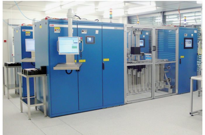
Automated IGBT and diode dies test system
